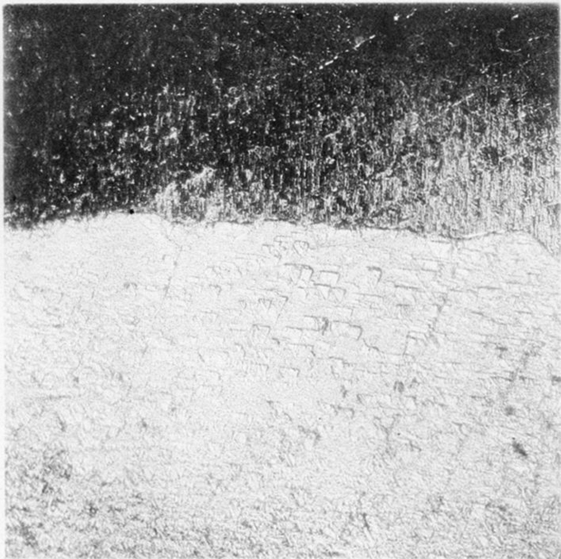
Fig. 29.—Tin-plate, etched. \times 100 .
