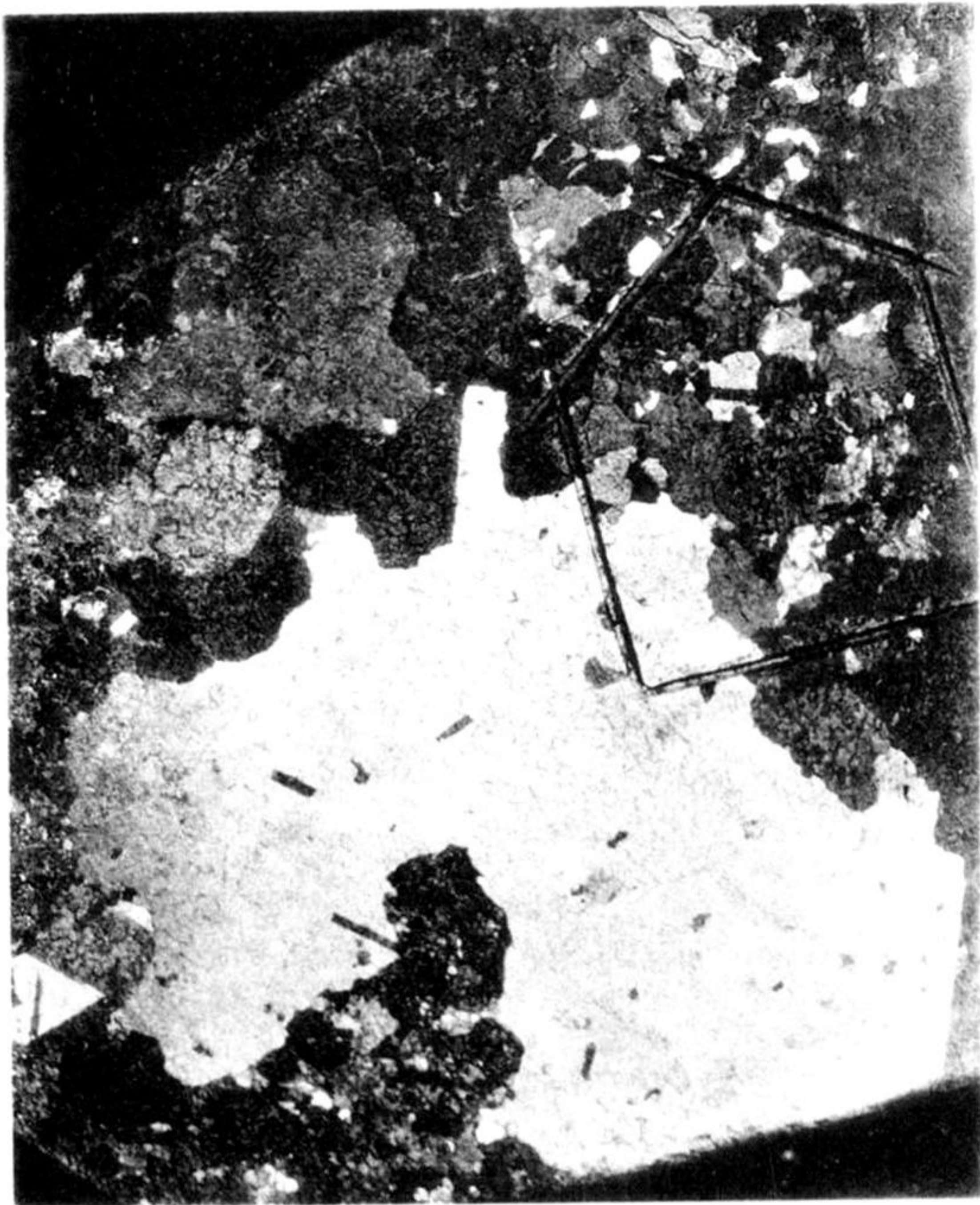
Fig. 26.—Same specimen as Fig. 25 (after 40 days at 200° C.) with incidence of light altered. \times 8 .
