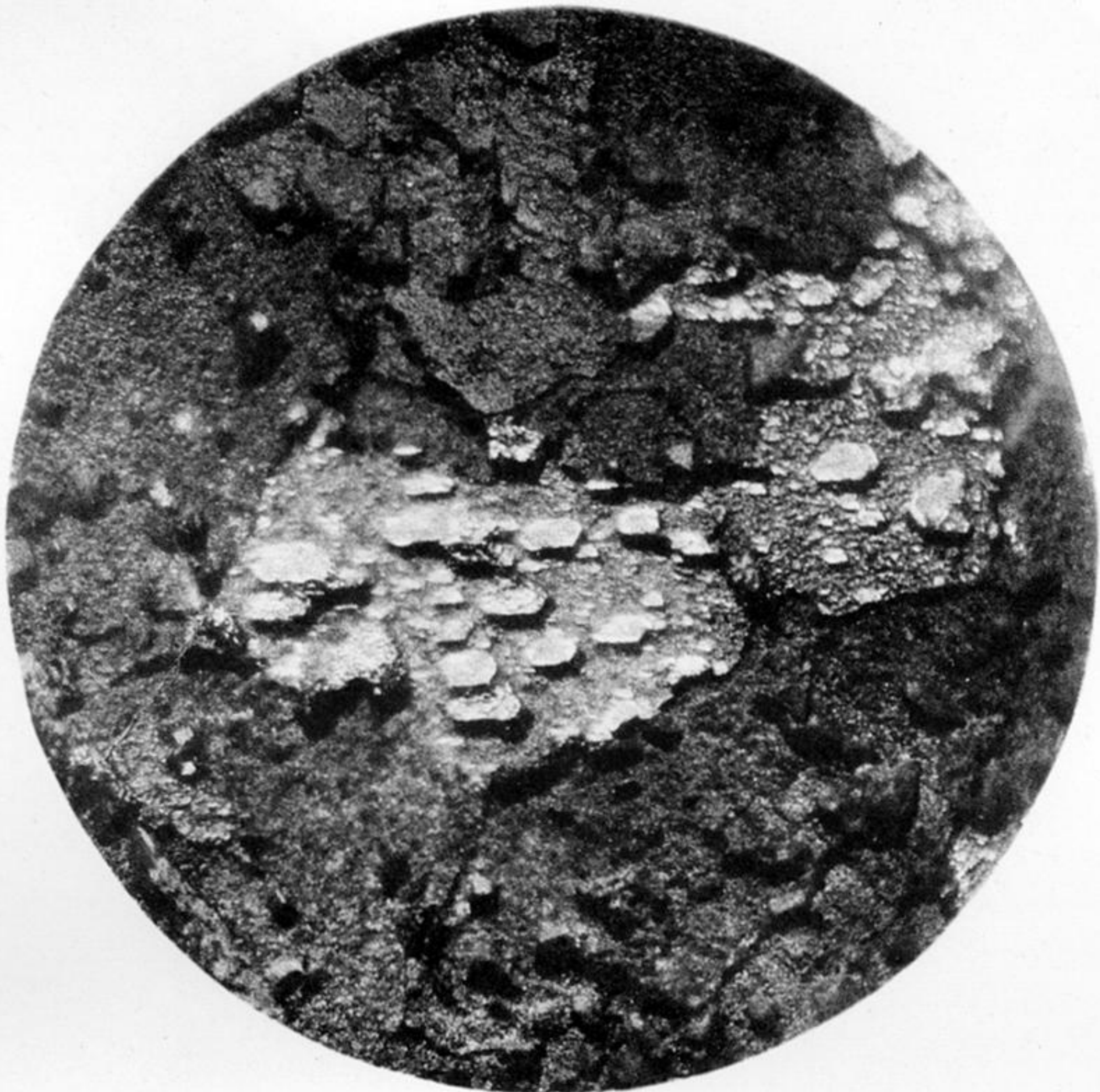
Fig. 5.—Etched sheet-lead. \times 100 .
